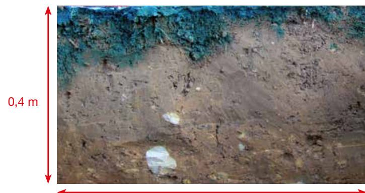
Entry of water into the soil profile in a field without barley seeds as secondary crop
