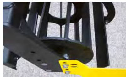
Crumbling bar behind the front roller 4
