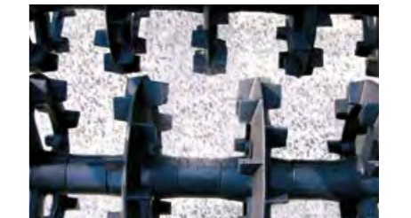
Rear crumbling rollers 7
